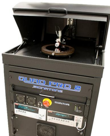
**QuadPro2 Resistivity Test System**
