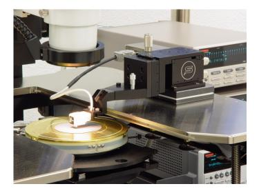
Sheet resistance mapping of thin films with a collinear 4-point probe (photo left)
