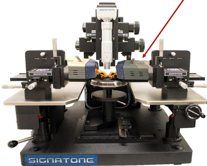
Micropositioners are available to hold virtually all the current models of Frequency extenders and tuners modules so that the module and the probe are moved and positioned as a unit (together). In this way, total ease of positioning can be achieved with minimum insertion loss.
