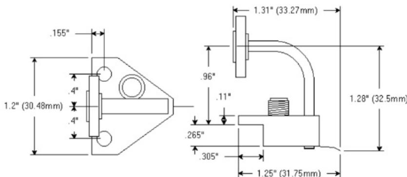
Model SP-90BT Waveguide Dimensions
