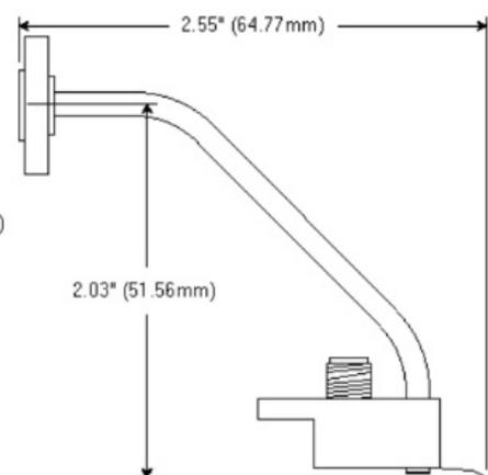
Model SP-90BT-M Waveguide Dimensions
