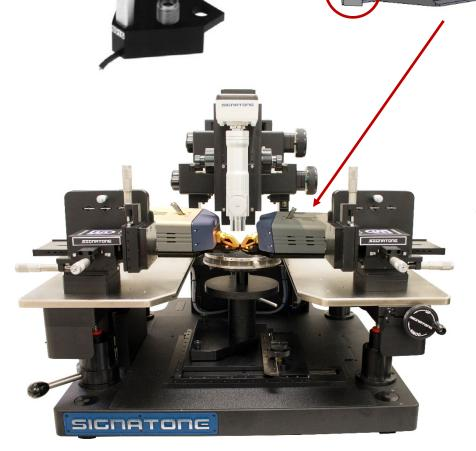
Signatone S-LAP-90 Large Area Positioner for mounting 50-1100GHz probes directly to the Frequency Extender with wave guide.
