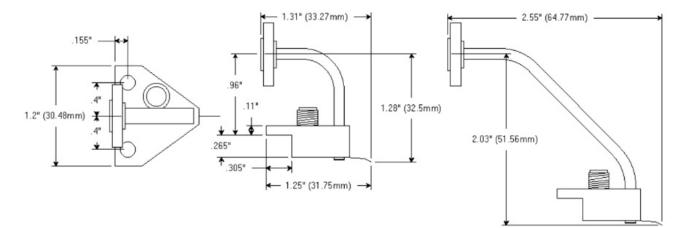
Model SP-220BT Waveguide Dimensions
