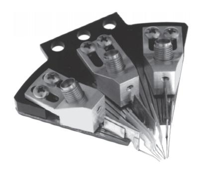
Sample: Multi-Contact Wedge with three 40 GHz probes and five dc needles
