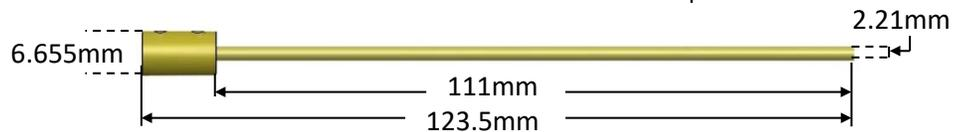
The Probe Mount Adapter Shaft is made out of Brass and is used to extend the Signatone Ceramic Blade Probe from the positioner. The Shaft may be bent or cut to the desired shape and length.
