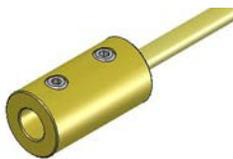
The Probe Mount Adapter Collar has a 3.22mm diameter hole for insertion of the Ceramic Blade Probe Mounting Post. Included are 4 very small (# 2-56) set screws for securing the Post in the Collar
