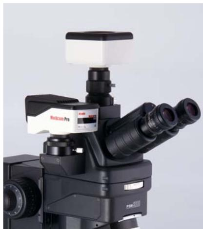
2 CCD Camera on dual Ports
