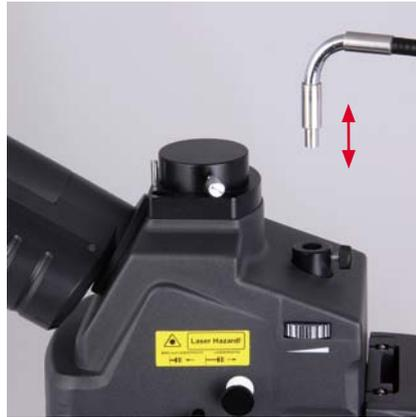
150W Halogen fiber optic with light guide and color temperature adjustable from 500K~3700K
